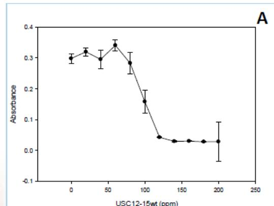
Figure 1. Graph showing the inhibition of microbial growth with increasing concentration of USC polymer biocide
